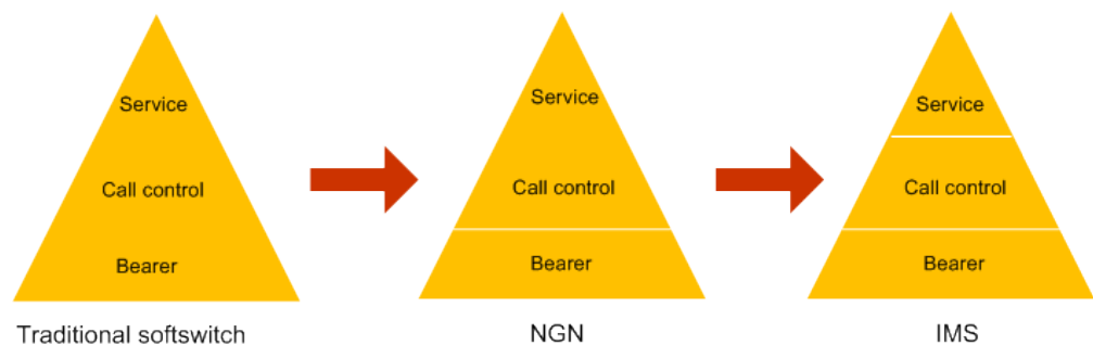
Figure 23-4 Control, bearing, and service separation
