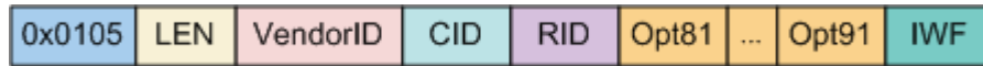
Figure 27-15 General format of a PPPoE packet carrying a vendor tag in PITP P mode
